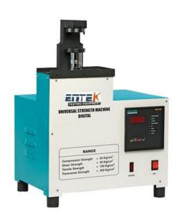
**SPECIFICATIONS**: Suitable For Compression Strength, Shear Strength, Tensile Strength, Transverse Strength With The Help Of Attachment, Capacity 50 Kg/Cm2 On Compression Scale With Motorized Loading Mechanism, Load Cell, Digital Strength Indicator And Compression Pads with computer interface with memory. **Attachments**:
